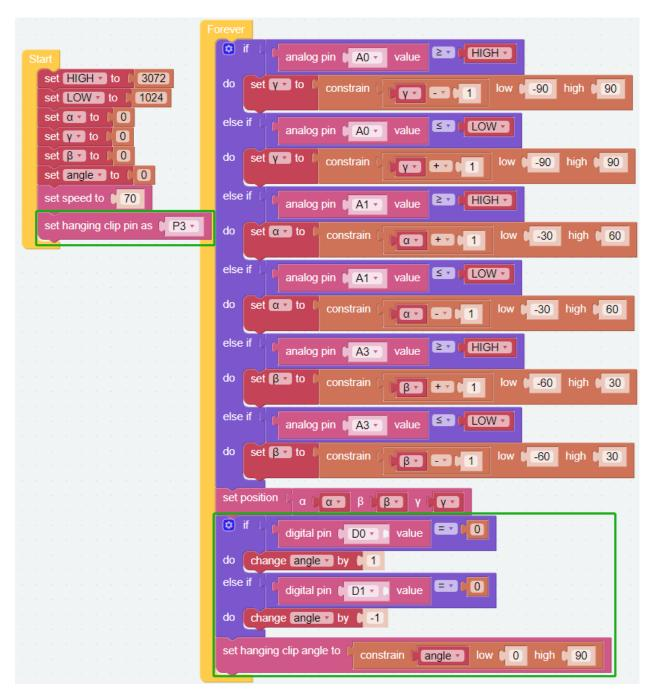
After the code is run, you can use the dual joystick module to control PiArm's arms and vertical clips at the same time. But you need to install *Hanging Clip* to PiArm first.
